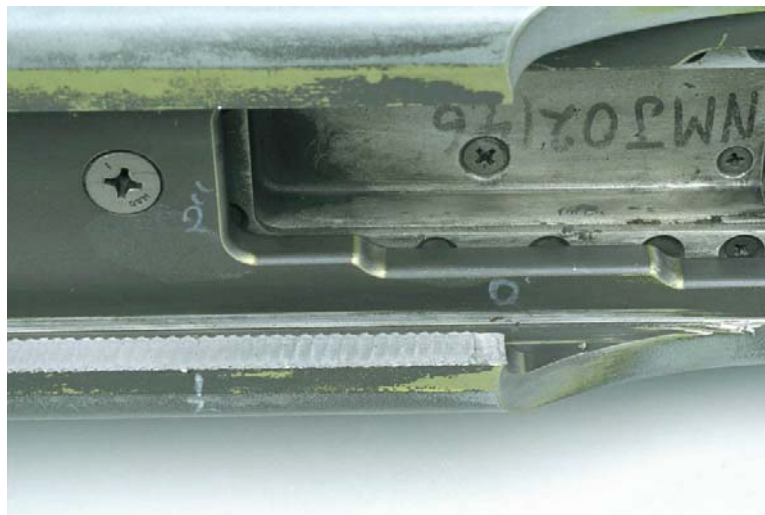
Figure 8: Rail 'Gouging' of the LAU-7 Launcher
