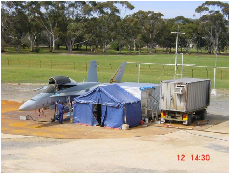
Figure 5: Implementation of Mini - Chamber Test Facility (MCTF) on the OATS
