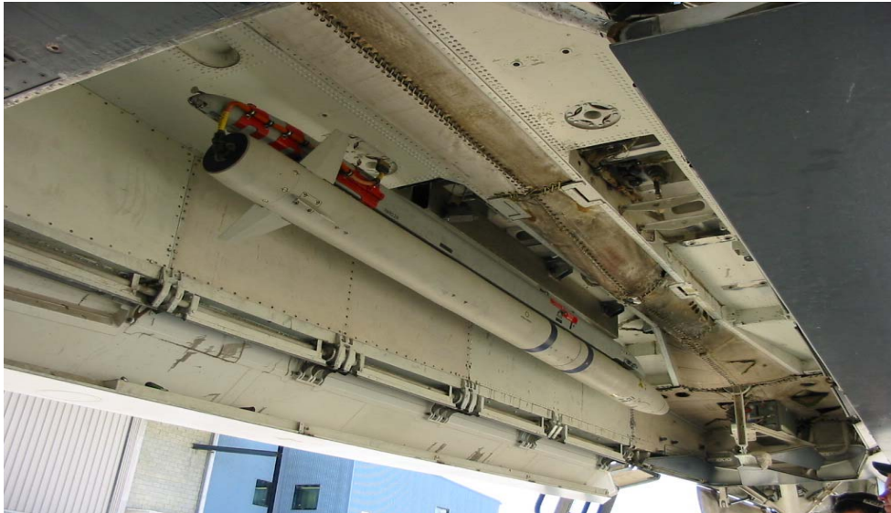
Figure 1: AIM-132 Advanced Short Range Air to Air Missile (fitted in the F-111 Bomb Bay)
