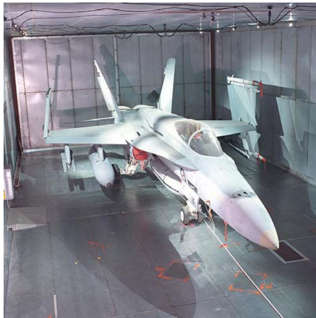
Figure 3a: F/A-18 Positioned in the DSTO Reverberation Chamber (front view)
