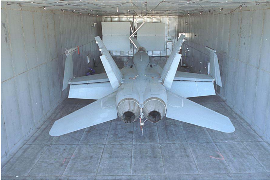
Figure 3b: F/A-18 Positioned in the DSTO Reverberation Chamber (rear view)
