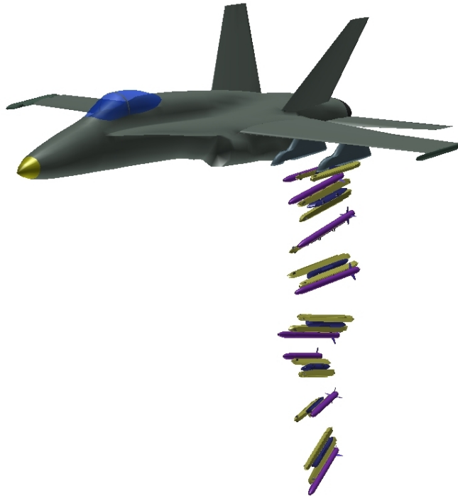
Figure 9: Simulated Jettison of the MLA in the Asymmetric Configuration
